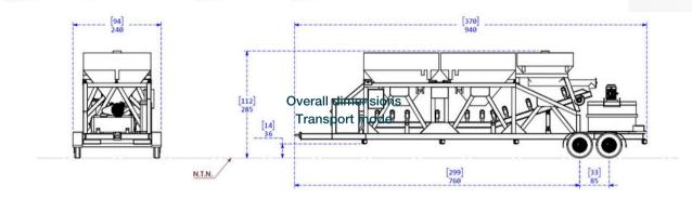
Dimension: centimeters (inches) N.T. N.: natural terrain level
